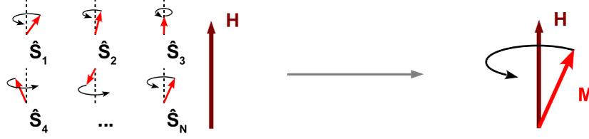
**Figure 2.1.:** In the context of the macrospin model, a large set of quantum mechanical spins  $\hat{S}_i$  (left) is treated as a single macroscopic magnetic moment  $\vec{M}$  (right), which precesses in the external field  $H$ .
