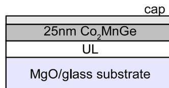
**Figure 3.21.:** Layer stacking for  $\text{Co}_2\text{MnGe}$ .
